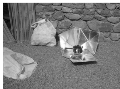
Figure 3 Demonstrating how a solar cooker made from cardboard and aluminium foil works in the village of Hathin. Photo Nadia Manasfi
